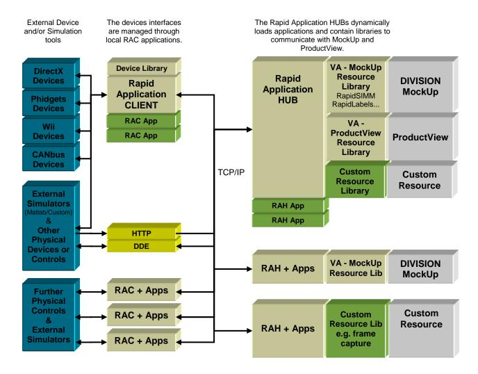
RAC Device libraries and RAH Resource libraries are embedded with the RAC and RAH run-times. RAC and RAH Applications are typically loaded dynamically, although custom versions can be created to form a totally integrated solution for security and license management purposes. The VA-MockUp Resource Library is matched to MockUp plug-ins.
